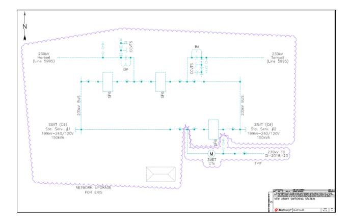
Figure 2 – Preliminary One-line of the PI-2019-7 230kV Switching Station (Tap on the Hartsel–Tarryall 230kV Line)
